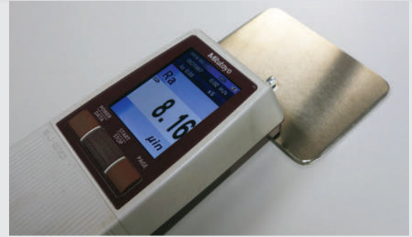
A profilometer (RA meter) is used to measure the roughness average of peaks and valleys in stainless material.
