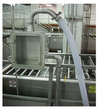
The integration of a vacuum sample system in a Mixer Blender is an efficient way to take product samples. There is no need for equipment and production stops because the vacuum sampler is automatic and can be delivered at different intervals to provide a true test of product consistency.
